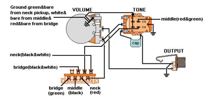
Note: Tailpiece should be connected to common ground.
