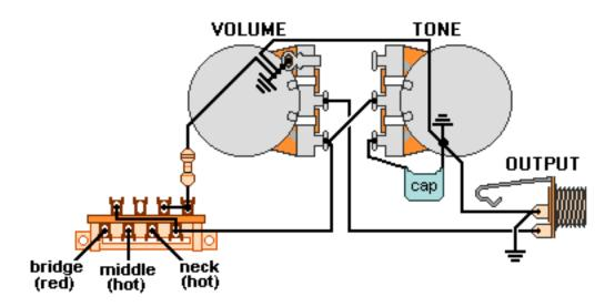
All other pickup wires not shown or mentioned go to ground. Note: Tailpiece should be connected to common ground. All grounds 🛓 must be connected.
