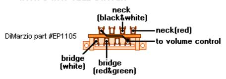
All other pickup wires not shown or mentioned go to ground. Note: Tailpiece should be connected to common ground. All grounds 🛓 must be connected.
