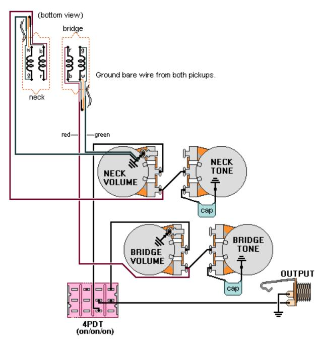
All other pickup wires not shown or mentioned go to ground. Note: Tailpiece should be connected to common ground. All grounds 上 must be connected.
