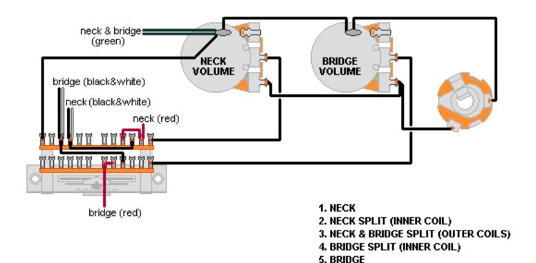
(Both pickups should be placed in the same direction...cables towards the controls.)
