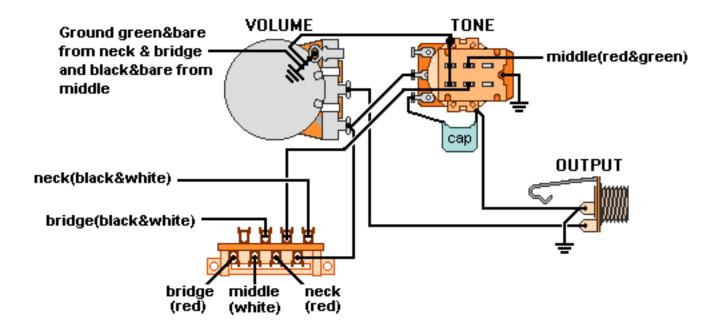
Note: Tailpiece should be connected to common ground. All grounds 🛓 must be connected.
