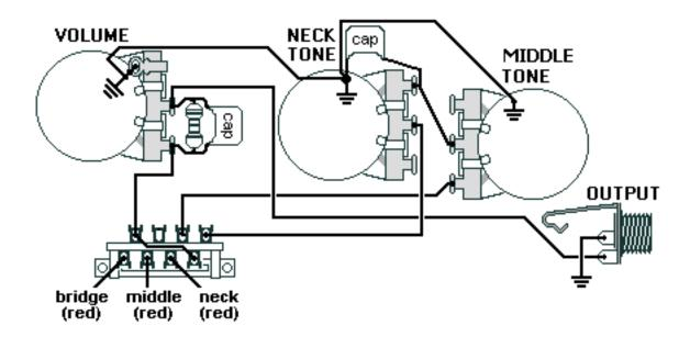
For each pickup, solder black & white together and tape connections. Ground green & bare wires.
