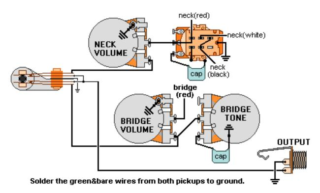
For bridge, solder the black&white wires together and tape up the connection.
