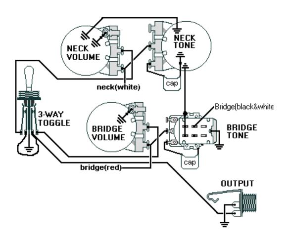
All other pickup wires not shown or mentioned go to ground. Note: Tailpiece should be connected to common ground. All grounds <u>L</u> must be connected.
