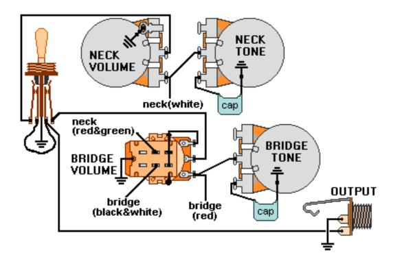
Ground black & bare wires from neck pickup and green & bare from bridge pickup.
