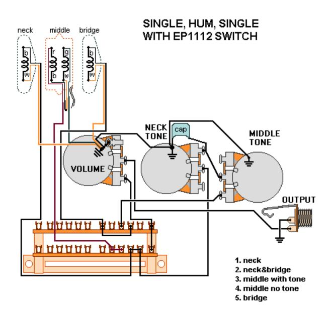
Note: Tailpiece should be connected to common ground. All grounds 🛓 must be connected.
