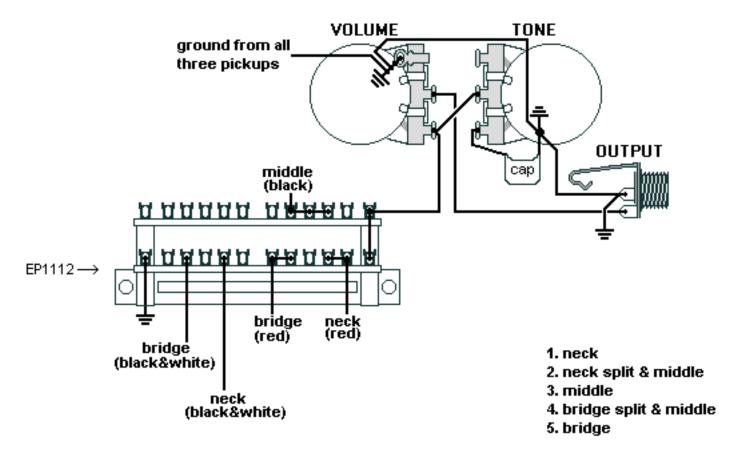
Note: Tailpiece should be connected to common ground. All grounds 🛓 must be connected.
